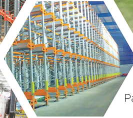
Push Back Pallet Racking
