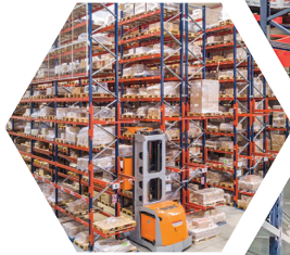
VNA Pallet Racking
